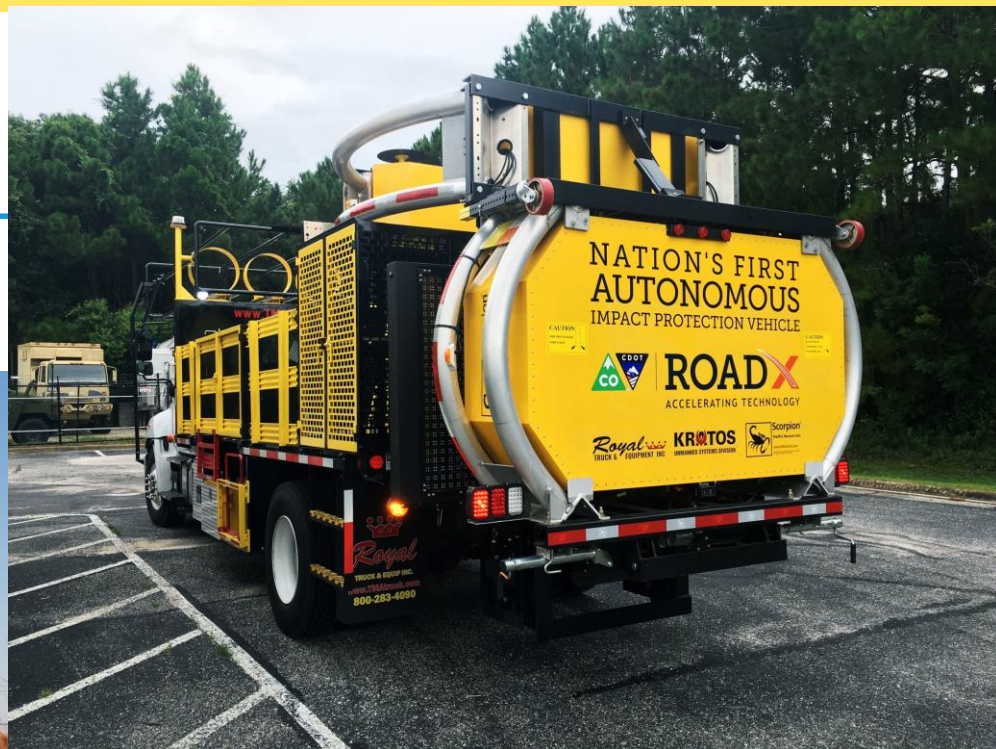
CDOT Automated Truck Mounted Attenuator
