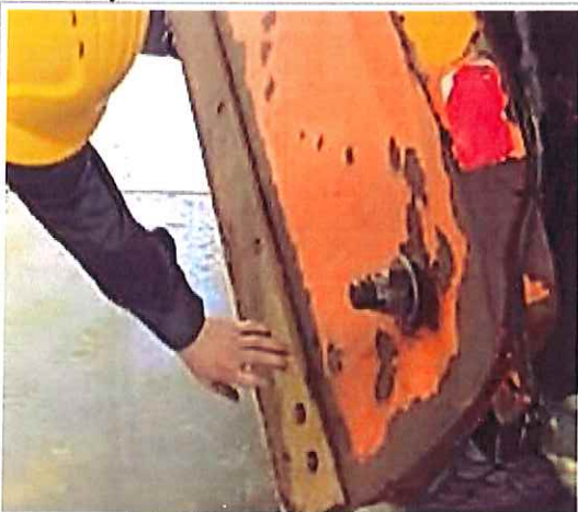
Uneven wear on wing-plow blade.
