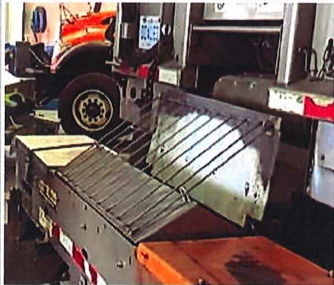
The Clumpinator tilts to eject objects caught in screen.
