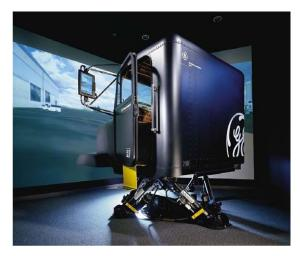
Figure 8. Mark II Motion-Based Simulator Used in Utah DOT Study (Source: Utah DOT, November 2004.)
