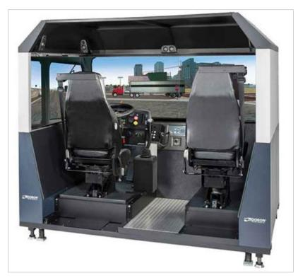
Figure 5. Doron SP660 Snowplow Simulator (Source: Ohio DOT, February 2022.)
