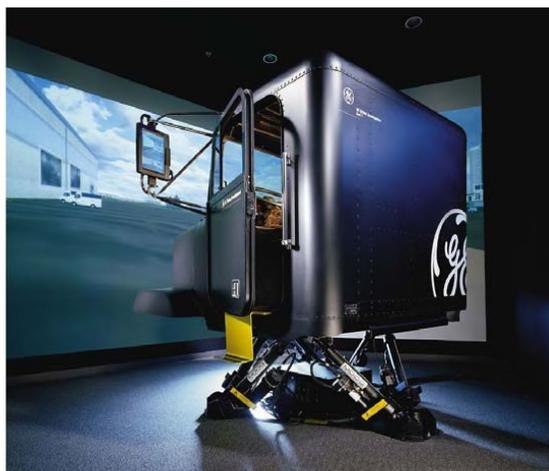
**Figure 8. Mark II Motion-Based Simulator Used in Utah DOT Study**
