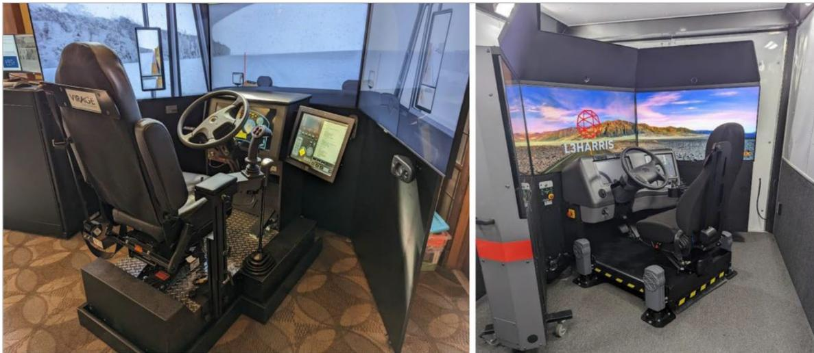
**Figure 4. Snowplow Driving Simulator Installations from Virage (left) and L3Harris (right)**
