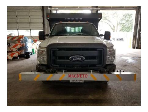
To unlock, the two pins are removed allowing the magnet to fold down into the working position.
